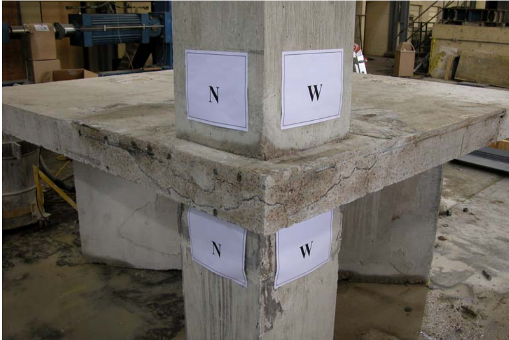
Figure B.4: Failure surface of Specimen LG1.0.
