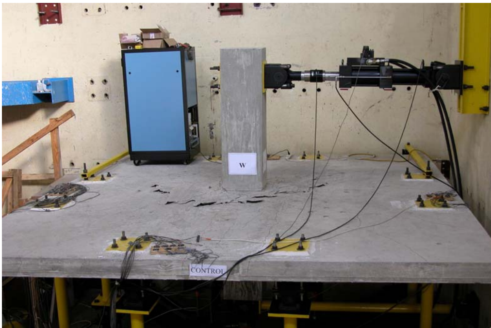
Figure 3.19: Failure pattern of Specimen L0.5.
