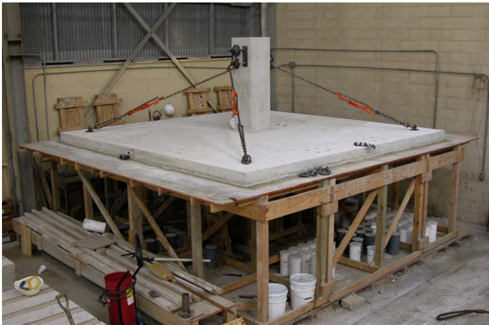
Figure 2.32: Preparation for specimen lifting.
